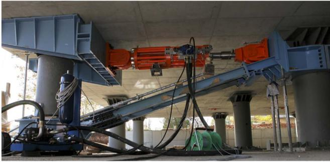
Fig. 9. In situ testing of an isolated building in L'Aquila.
